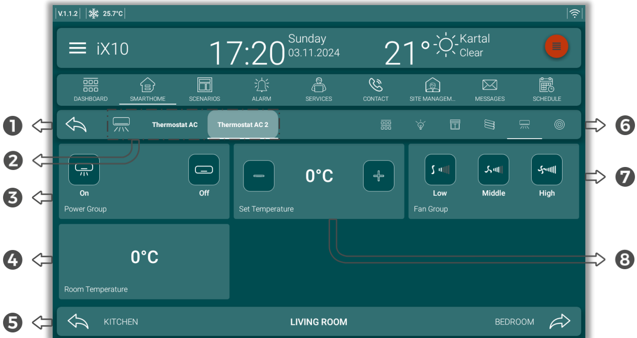
Fig. 20: Air Conditioner Section
